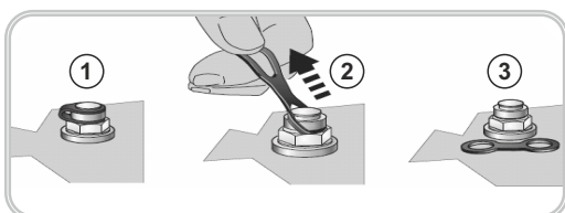
Figure 3: Activation of Vent Plug
